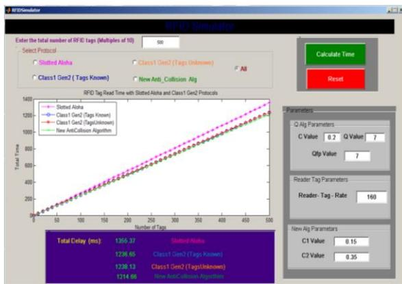
Fig.10. RFID Simulator Interface for All Algorithms, With 500 Tags
