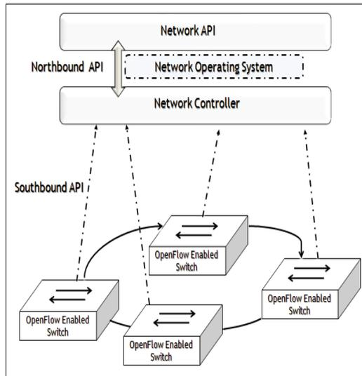
Fig.2. Simple SDN Architecture
