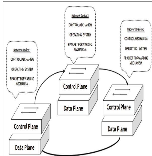
Fig.1(b). Control and Data planes in Software Defined Networks
