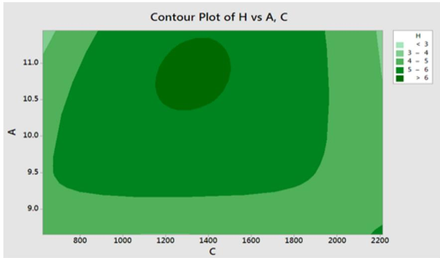
Fig. 7. Contour plot of burr height with respect to drill diameter & spindle speed
