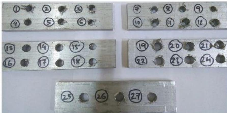
Fig.2. View of the work piece after drilling.[21]
