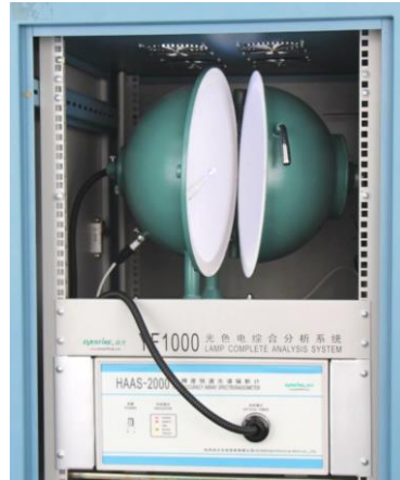
Fig. 3. Photograph of the complex for measuring the parameters of LEDs.
