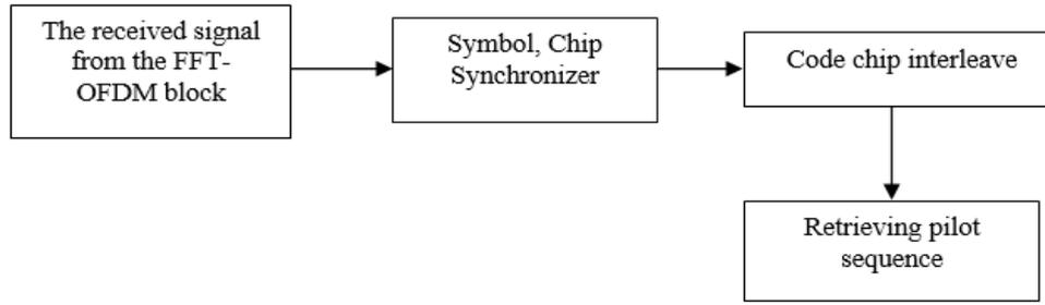
Fig.4. Pilot decoder block.
