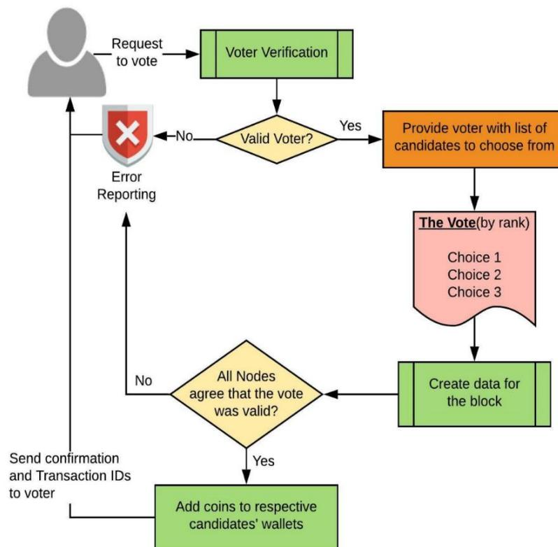
Fig.3. Flow of system control for the proposed voting mechanism
