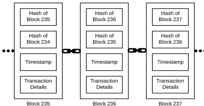
Fig. 6. Hashing mechanism imparting security to blockchains
